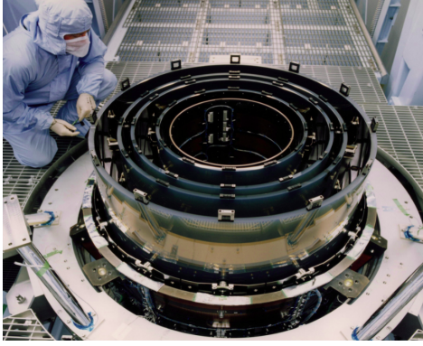
(a) The 4 nested thick mirrors of the CHANDRA telescope.
